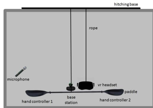
**Figure 2.** Installation in real space.
