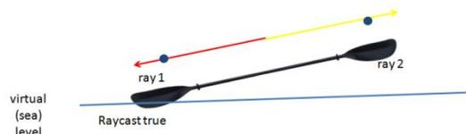
**Figure 3.** Raycasting mechanism identifying the paddle colliding with the virtual (sea) level.
